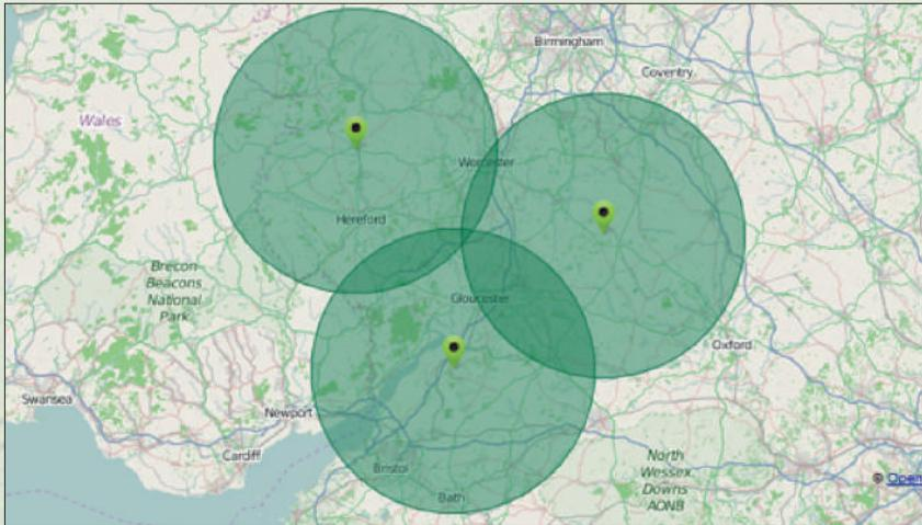
Above map shows the current extent of the TAG RTK network, using the three RTK Base Stations sited at Leominster, Dursley and Blockley. The green rings show the 40 Kilometer radius of RTK signal coverage. The correction signal is picked up by a sim card in the machine-mounted RTK modem providing repeatable accuracy.
