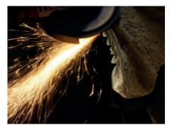
Hand-held grinders are not the best way to sharpen blades of any kind! Overheating leads to blade failure, while incorrect grind angle can cause increases of fuel by up to 30% compared with correctly sharpened knives/blades.
