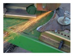
Professional sharpening system at TAG, means that baler and forage wagon blades and knives can be set-up and sharpened precisely for maximum cut performance, long blade life and best fuel consumption.
