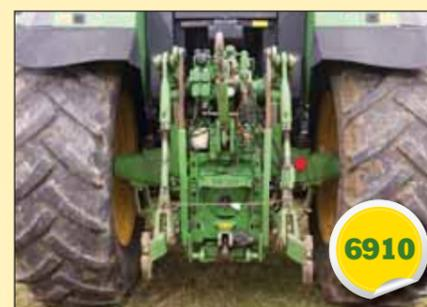
Maximum lift capacity of the John Deere 6910 isn't far behind the 4755 and 7710 models at a useful 7699kg. Like the 7710 it has electronic lower link sensing. Push-back pick-up hitch provides a good view of the hook when coupling-up to trailed kit.
