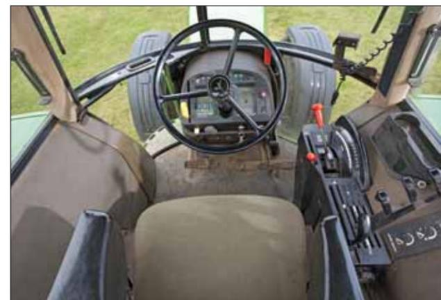
**Above: Both of the 4755s are fitted with near-identical SG2 cabs. Old-school interior looks Spartan by today's standards, but back in the 1980s and early 90s it was one of the ultimate operator stations. All the essential information is displayed by the IntelliTrack monitoring system with LCD readouts, a new feature that was introduced with the 55 Series in 1989.**
