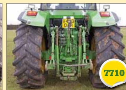
Muscular rear end of the farm's John Deere 7710 provides a maximum lift capacity of 8150kg (or 5650kg when measured 61cm behind the hitch points). Other features include three SCVs with pressure-release couplings and a heavy-duty Dromone hitch.
