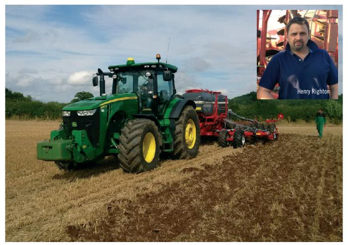
The Focus TD's tine cultivation frame can be quickly and simply released from the chassis at four mounting points. Once taken from under the machine, it can easily be replaced with the DiscSystem with 52cm discs to create a compact rotary disc harrow, increasing the flexibility of the machine enormously.
