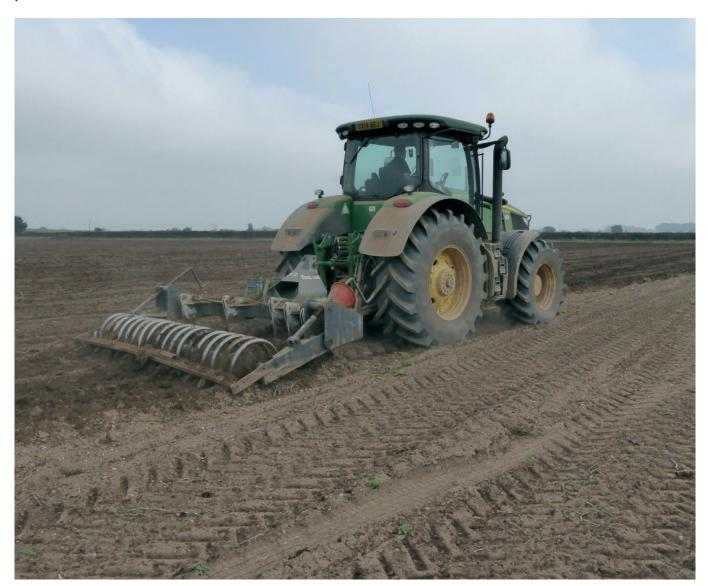
In addition to a large 6 furrow, variable plough – each furrow can plough up to 20 inches wide, Stephen Watkins employs heavy-duty cultivation equipment such as a 5 leg Flexicoil subsoiler and a 3 metre Simba DTX to maintain soil condition for all the specialist crop requirements., all of which the 7250R with its AutoPower Transmission, is more than capable of working.
