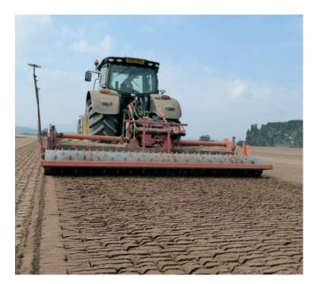
Stone burying at 0.4 km/h can be demanding for the operator, but Green Star Precision Farming technology from John Deere, means the 6210R tractor purchased from Tallis Amos Group, steers in a straight line, automatically avoiding overlaps.
