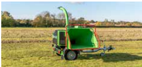
GreenMech's QuadChip 160 has a turnable in-feed that spans up to 270 degrees of angled adjustment
