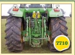
Muscular rear end of the farm's John Deere 7710 provides a maximum lift capacity of 8150kg (or 5650kg when measured 61cm behind the hitch points). Other features include three SCVs with pressure-release couplings and a heavy-duty Dromone hitch.
