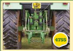
Back-end of the John Deere 4755 looks positively skinny compared to the 7710. This is not surprising since the 4755 was the final iteration in an evolutionary process that began with the 'New Generation' Deeres in the 1960s. Maximum life is still a useful 8400kg.
